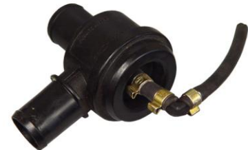
Original, worn out Bosch® boost shut-off valve
